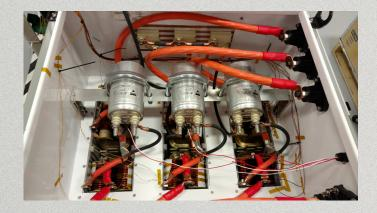
JDES developed this rapid prototype using a standard electrical cabinet and JDES technology. This project included electrical design to define and select the passive filter components, mechanical expertise for high power packaging and high power density water cooling, and production AC supply software inside the inverter.
